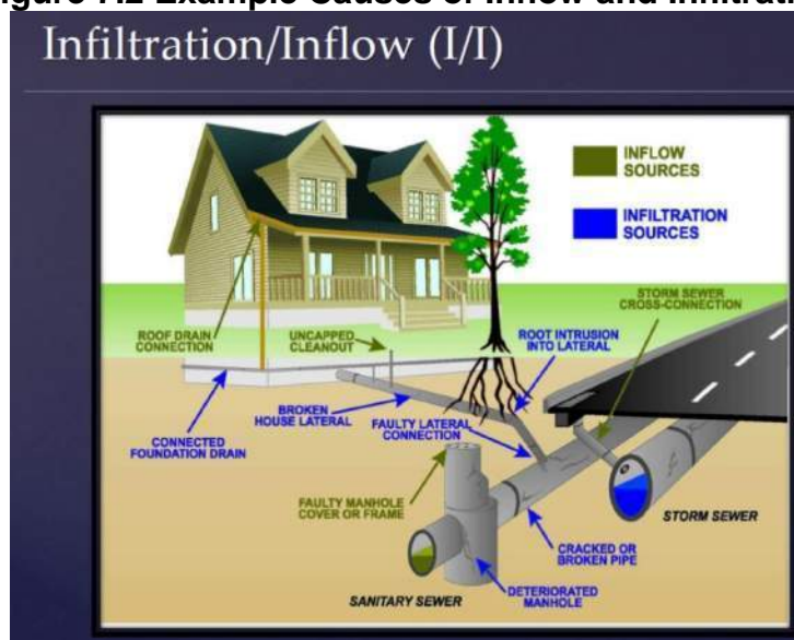
Figure 7.2 Example Causes of Inflow and Infiltration
